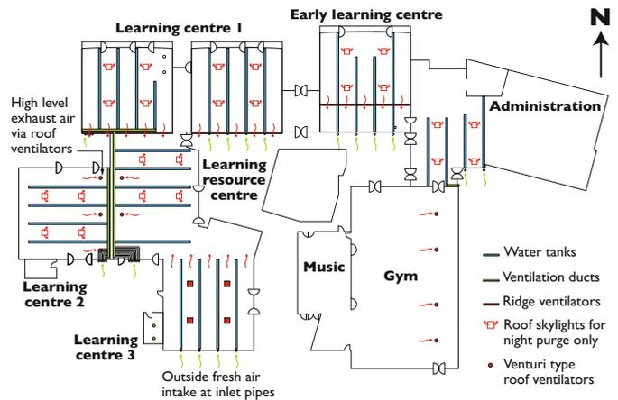
The plan form of Meadows Primary School showing the arrangement of water tanks beneath the structural concrete slabs, the four structural columns per 17 sq m building module (shown in the learning centre to the south), and the rooflights in the other modules.
