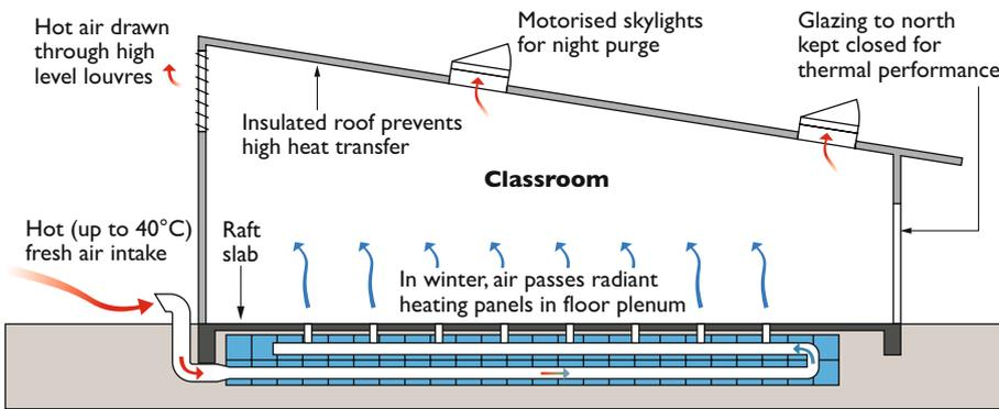
Cross-section of a typical classroom module and water tank, showing the operating condition for the summer months. The air intakes will be from large funnels feeding into a slightly enlarged (375mm) pipe. Fabric airtightness will be crucial for ensuring that the supply air traverses the air ducts rather than short-circuits through intentional and unintended gaps in the facade.
