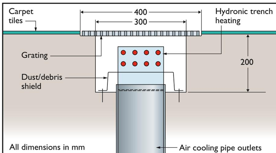
A cross-section through the trench heating system, based on four groups of twinned copper pipes run in ventilation channel recesses.
